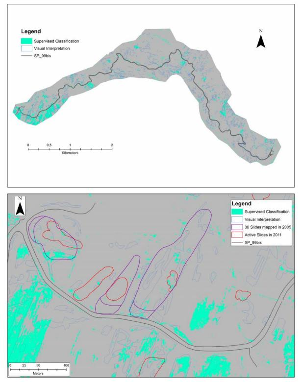
Figure 3:(Upper) Distributions of wet areas in March 2011 on slopes traversed by SP\_99bis road, from supervised classification and from visual interpretation;(Lower) Close-up of the westernmost part of the Upper figure showing also major 2005 landslides and landslides active in 2011.
